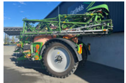
Amazone UX3200 - 2015 24m Boom, 3600 Lt Tank Plus 320 Lt Tank
