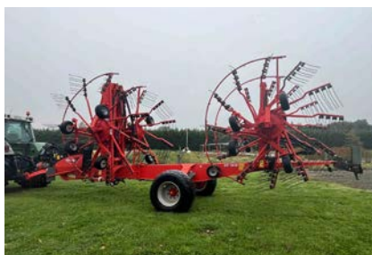
Kuhn GA13131 Rake 2016, 4 Rotor, ISOBUS, hydraulically driven rotors
