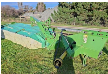
Krone ECR 320 Mower EasyCut 3.2m Mower, Gear driven, Centre of gravity suspension
