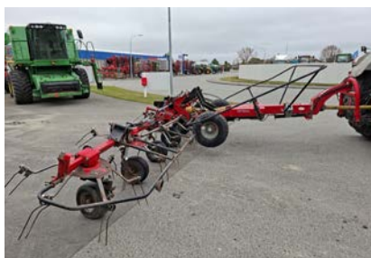
Massey Fergusson TD1649 Tedder 8.6m working width, 6 rotors
