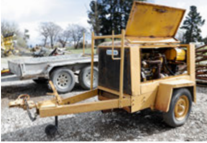
Broomwade Air Compressor
